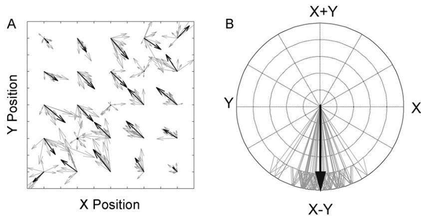
**Fig. 9.** Bootstrapping of vector fields. (A) Vector field described by Eq. (7) (black vectors) with simulated bootstrap-resampled versions of the same field superimposed (grey vectors). (B) Field orientations for the 'mean' field in A (black) and the bootstrapped fields (grey).
