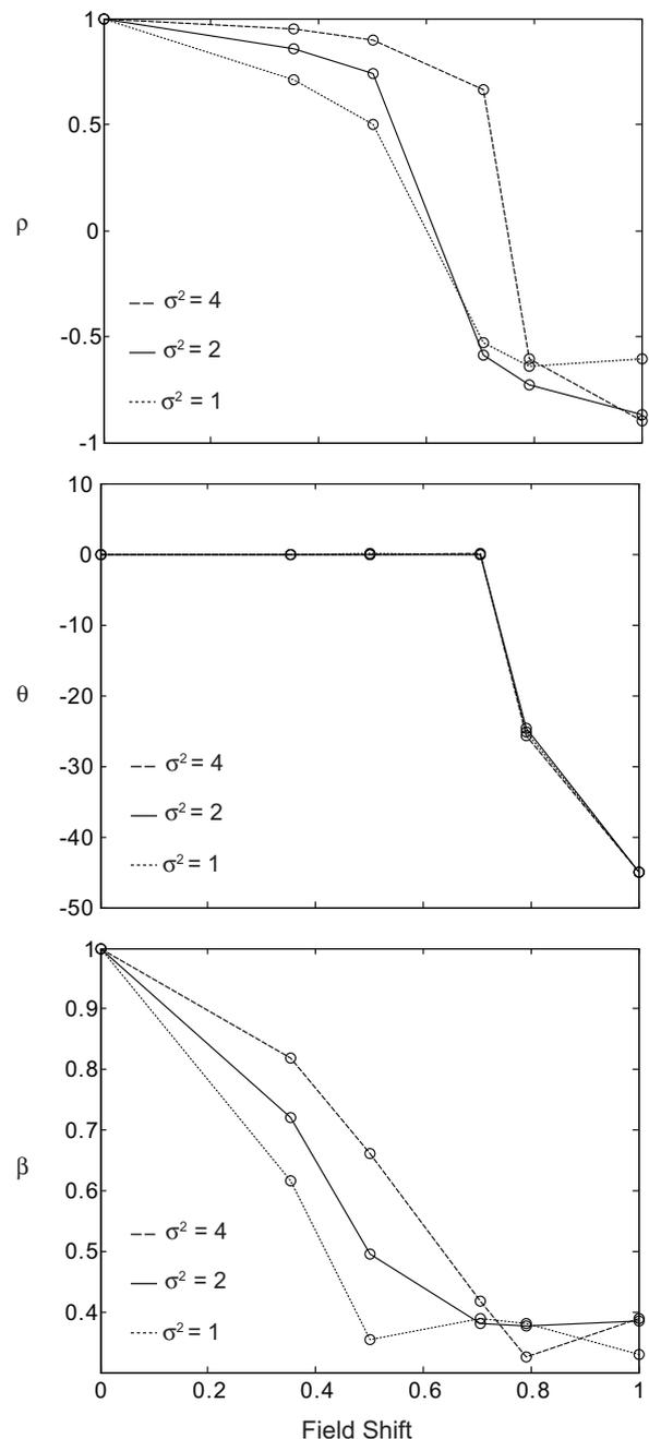
**Fig. 5.** Variation in vector correlation parameters with response field shift. Data for 2D Gaussian response fields of various widths are shown. Field shift is defined as the norm of the vector joining the peak of a shifted 2D Gaussian with an identical 2D Gaussian located at the center of the workspace.
